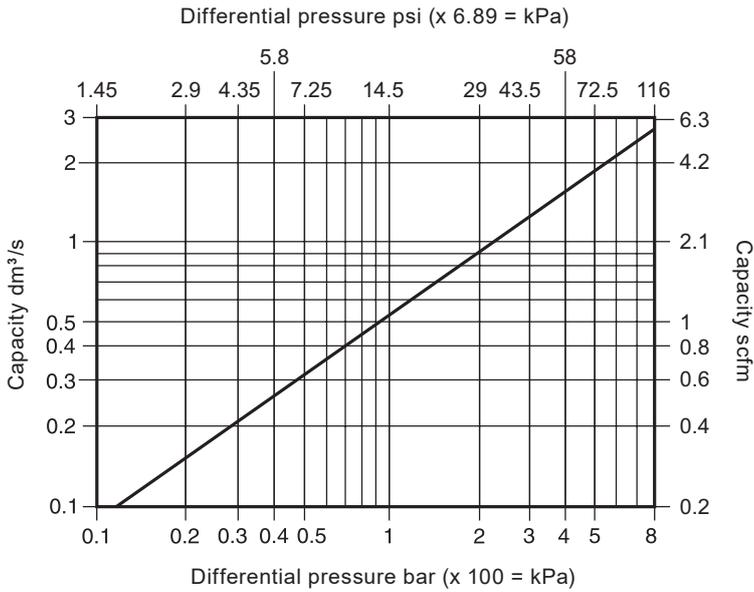
If the temperature of the air differs from 16 °C, the discharge capacity from the graph can be corrected by multiplying it by the following equation:
