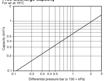
If the temperature of the air differs from 16°C, the discharge capacity from the graph can be corrected by miltiplying it by the following equation:
