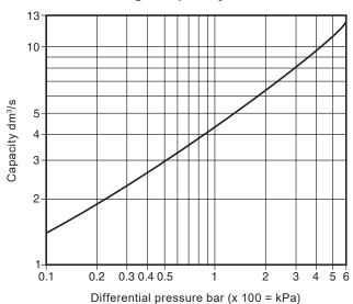
If the temperature of the air differs from 15 °C, the discharge capacity from the graph can be corrected by multiplying it by the following equation:
