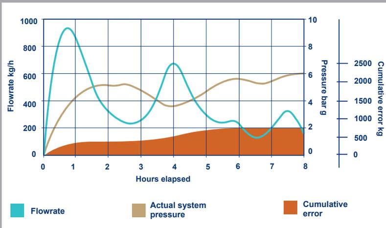
In the example above, a simple non-compensated flowmeter is set for 5 bar g. The actual pressure in the system varies through the day and unless this is allowed for, by the end of the day, very significant errors can arise. This can be avoided with a density compensating meter, such as the TFA.
