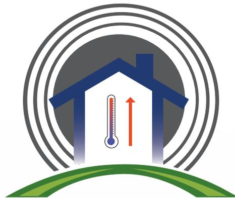
As the outside weather temperature reduces the temperature in the heating system is increased.
