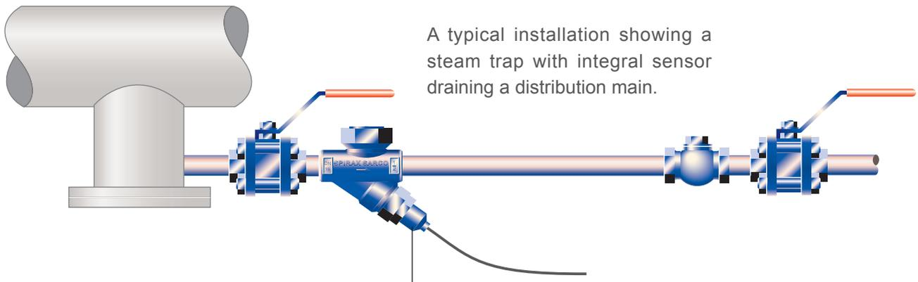
The steam trap is fitted with a Spiratec sensor, which can be checked manually or automatically.
