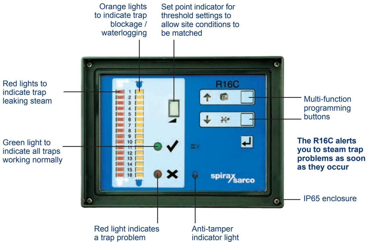
The R16C steam trap monitor is available for 90 - 240 Vac or 24 Vac supplies and for either wall mounting or panel mounting. The box is ABS plastic and has an IP65 enclosure rating, when fitted with suitable cable glands.
