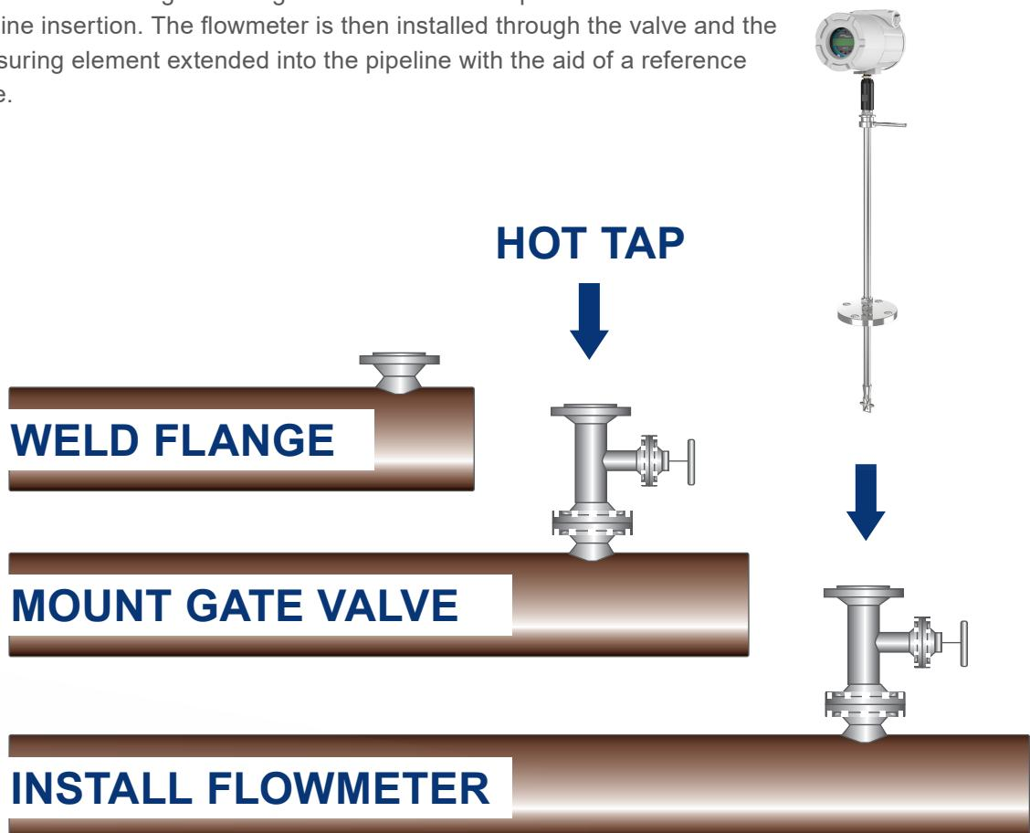
As the RIM20 can be fitted directly into operational pipework, installation is quick and easy without process shutdown. The cost of labour is reduced and data can be gathered more swiftly. Typical savings can be as much as 80% for DN600 pipelines and 50% for the DN250 pipelines.
