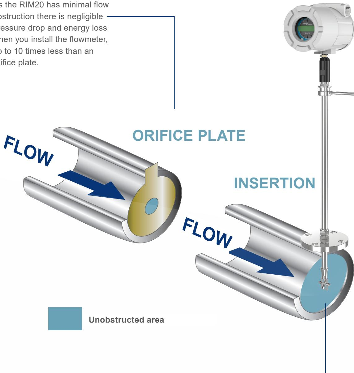
The insertion probe occupies a small area, leaving most of the pipeline unobstructed. Because it has a low pressure drop it is very efficient and flow pressure remains high.
