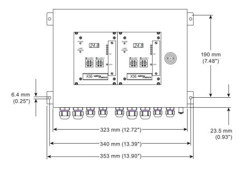
Fig. 7 Dimensions with wall mount housing S19-42 stainless steel 1.4301/SS304 - IP65
