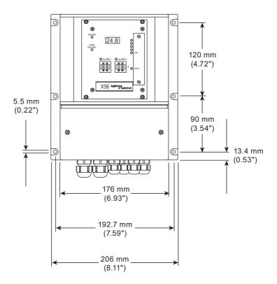
Fig. 5 Dimensions with wall mount housing B19-21
