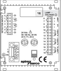
Fig. 19 Potentiometer for lamp voltage
