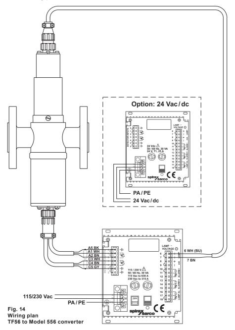
8.4.1 Wiring plan TF56 to Model 556 converter
