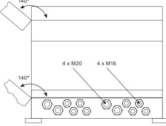
6.2.3 Dimensions for wall mount housing S19-42 -Stainless steel 1.4301 / SS304 - IP65 (option)
