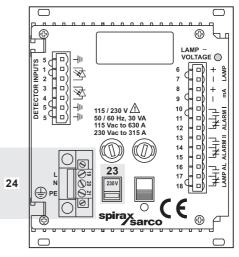
Fig. 11 Connecting the power supply 115 or 230 Vac
