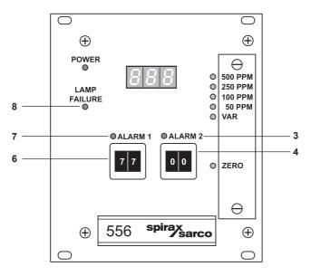
Fig. 22 LEDs and encoding buttons for alarms
