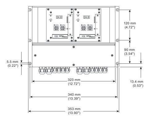
Fig. 6 Dimensions with wall mount housing B19-42
