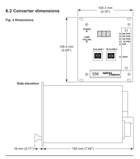
6.2.1 Dimensions for wall mount housing B19-21 -Plastic (ABS) - IP66 (option)
