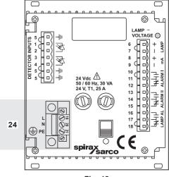
Fig. 12 Connecting the power supply 24 Vac/dc
