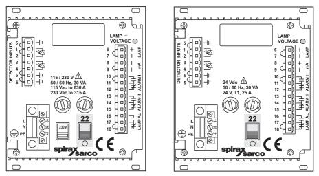
Fig. 18 Power switch on converter 115/230 V (left) and 24 V (right)
