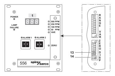
Fig. 23 Potentiometer for digital read-out adjustment
