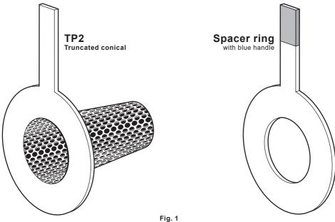
TP1, TP2, TP3 temporary cone, flat shaped strainers and spacer ring
