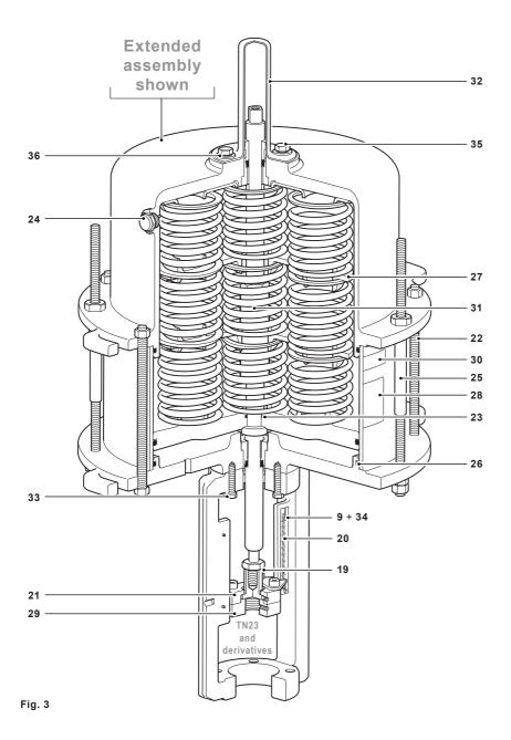
TN2000 Series Pneumatic Piston Actuators for DN125 to DN300 Spira-trol™ Series Control Valves
