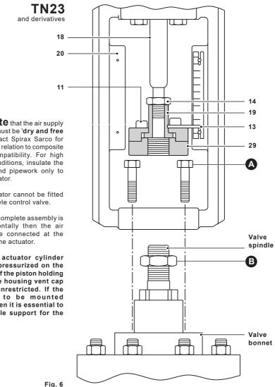
Please note that the air supply to the actuator must be 'dry and free from oil'. Contact Spirax Sarco for more details with relation to composite tube/media compatibility. For high temperature conditions, insulate the control valve and pipework only to protect the actuator.
