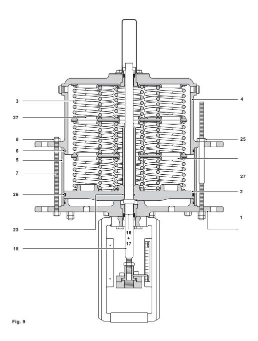
TN2000 Series Pneumatic Piston Actuators for DN125 to DN300 Spira-trol™ Series Control Valves spirax /sarco
