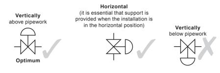
In an horizontal position, we recommend to use a support fixed to the threaded bar with an additional nut.
