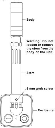
Warning: Do not remove the enclosure from the stem as this could cause damage or break the internal wiring.
