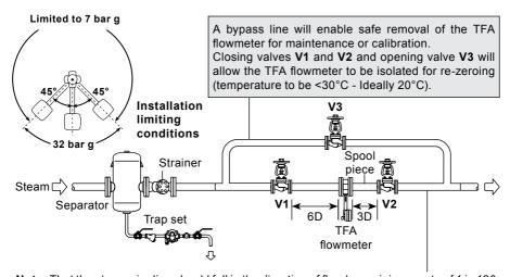
**Note:** That the steam pipeline should fall in the direction of flow by a minimum rate of 1 in 100.
