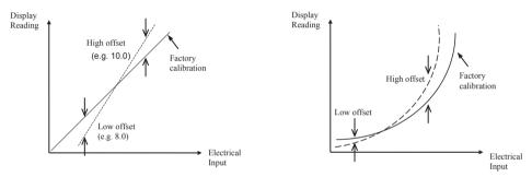
Two Point Offset Applied to Linear and Non-linear Inputs
