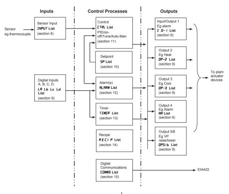
The Process Value 'PV' (temperature or pressure) is measured by the sensor and compared with a Setpoint (SP) set by the user.
