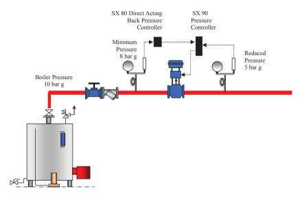
The SX90 remote setpoint limit will represent the downstream setpoint, 5 bar g The SX80 local setpoint will represent the upstream setpoint, 8 bar g
