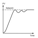
Autotune starts 1 minute after being turned on to determine steady state conditions.
