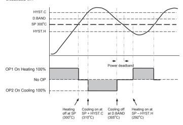
Heating and Cooling Type both on/off
