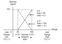
Lac. Land rEn. E may be used where two controllers are operated as a cascade pair. For example, one controller is controlling or limiting the steam pressure supply to a heat exchanger and the second is controlling the steam flow as a way to control the output temperature of the fluid being heated in the exchanger. A similar requirement occurs when two temperatures are cascaded.
