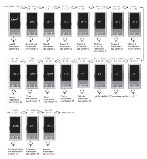
In SX80 controllers some lists are not available, for example Output 5, Output 6, and Digital Communications. In SX80 Logic Inputs A and B are available, Logic Inputs C and D are not available.
