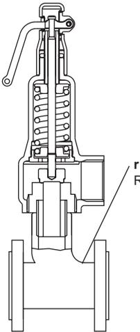
Radius 'r' not less than inlet diameter
