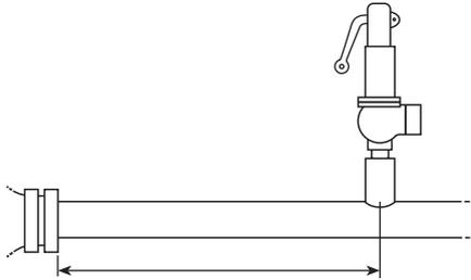
8 - 10 pipe diameters downstream of converging 'Y' fittings or bends.
