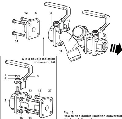
How to fit a double isolation conversion kit to a single isolation valve
