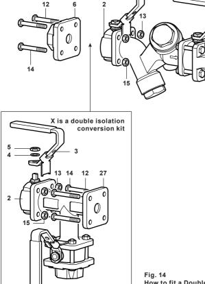
Fig. 14 How to fit a Double Block and Bleed conversion kit to a single isolation STS17.2
