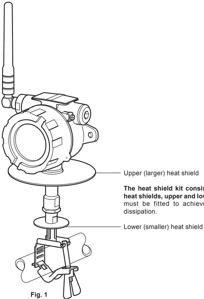
**Note:** The pictures below shows the STAPS head with the standard clamp used for small pipe sizes. The retaining nut arrangement is the same for all other types of clamp too.
