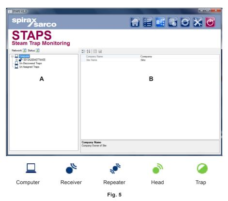
**Section A** in Figure 5 above shows the 'network tree' and indicates which Heads and Repeater are associated with which Receivers.
