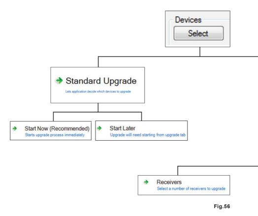
Standard Upgrade; the system will automatically review the network to identify which devices have older firmware and choose all Receivers, Repeaters and Head units that require upgrading. Custom Upgrade; this allows you the user to choose which units you would like to upgrade.
