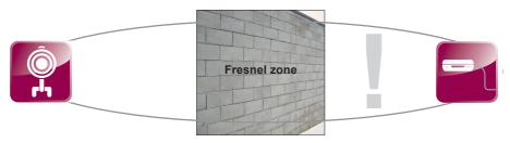
Fig. 5 Fresnel zone with blockage (obstacle) - Bad
