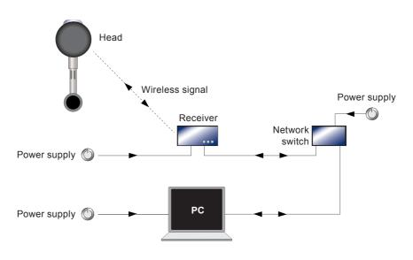
Fig. 12 System using network switch
