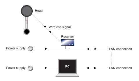
Fig. 11 System using building LAN (network)
