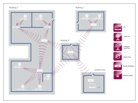
Fig. 3 Wireless architecture without access to LAN network
