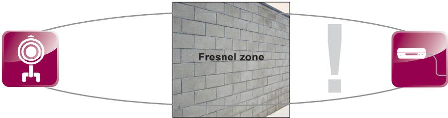
**Fig. 5 Fresnel zone with blockage (obstacle) - Bad**
