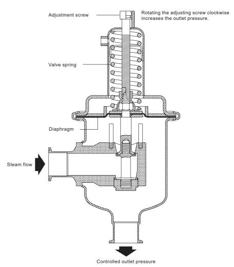
Fig. 3 How the SRV66HC works
