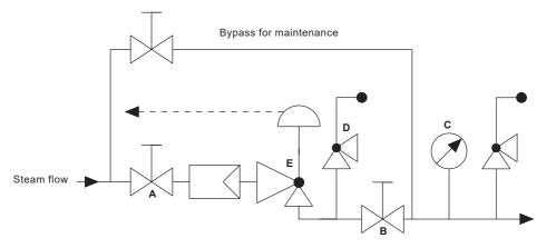
Fig. 5 Isolate the valve
