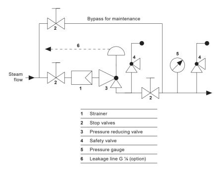
Fig. 2 Recommended installation
