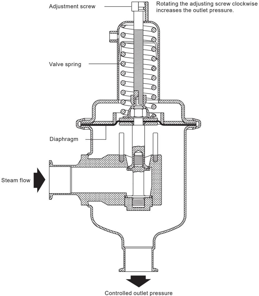
Fig. 3 How the SRV66HC works
