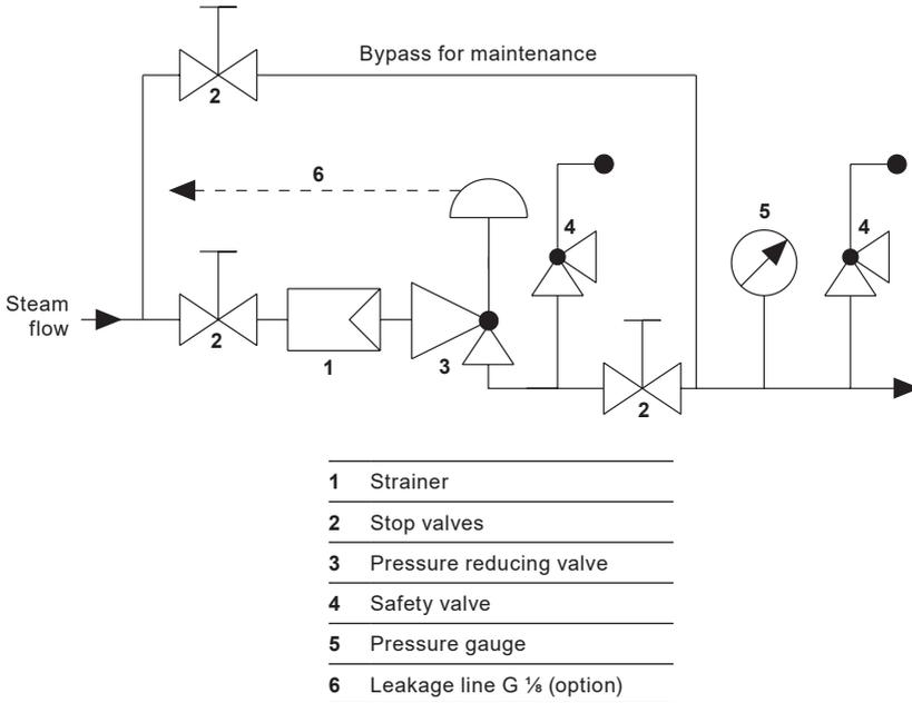
Fig. 2 Recommended installation
