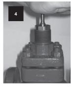
Firmly and briskly push the stem fully down.
