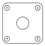
DN15 - DN50 bonnet tightening sequence
