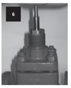
After each tightening sequence lift the stem fully.
