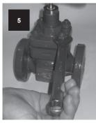
Using a torque wrench lightly and evenly tighten each bolt or nut by 45°, following the sequence illustrated in Figure 4, page 15.
