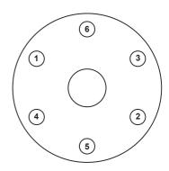
DN65 - DN100 bonnet tightening sequence
