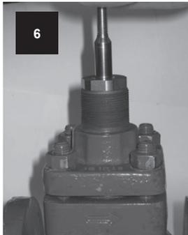
After each tightening sequence lift the stem fully.
