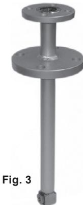
The spray nozzle desuperheater, type SND is an assembly which comprises one or more spray nozzles, cooling water inlet pipe, counter flange and cooling water inlet flange. The counter flange allows others to fit the SND onto a flanged branch in the steam pipework.
