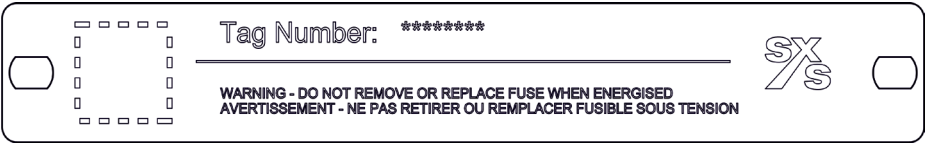
Fig. 4(c) Plate with measuring point tagging (Tag number)
