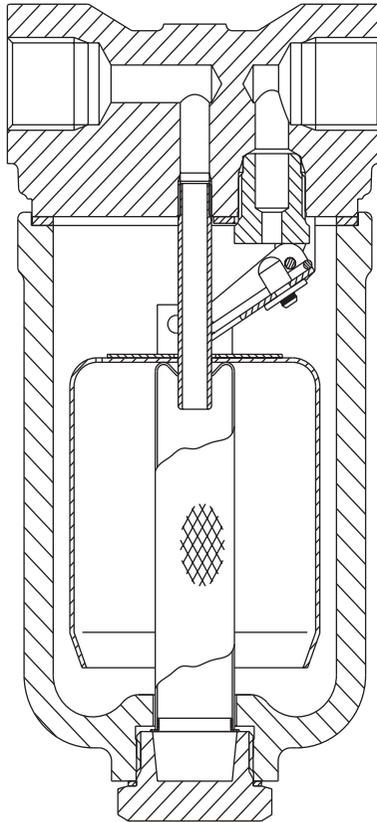
Fig. 1 SCA series inverted bucket steam trap
