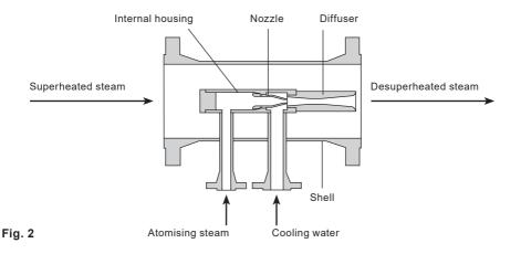
It can also be supplied with butt-weld ends (not shown) for welding directly into the steam line by others.
