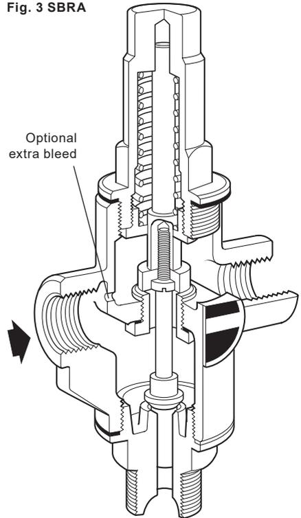
With KX and KY valves (DN32 - 50) (Figure 5) again models are available with or without bleed. Valves with a bleed arrangement have a 3 mm hole between the inlet and outlet. This permanent bleed arrangement can be sealed by tapping the hole and sealing it off with a 4BA or M4 screw before the valve is installed.
