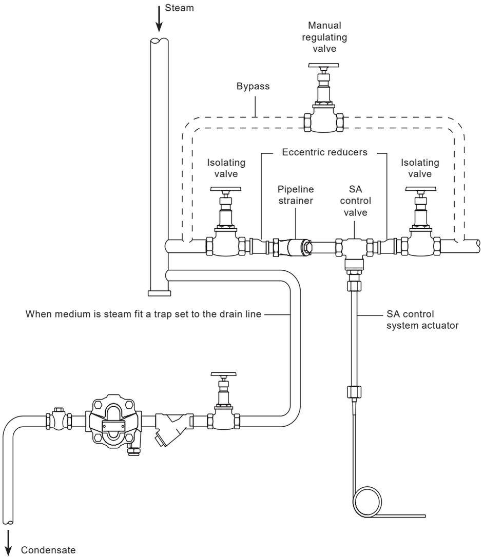
**Fig. 1 Typical installation showing recommended bypass**
