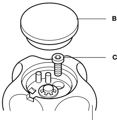
**Fig. 2** Adjustment head (knob)
