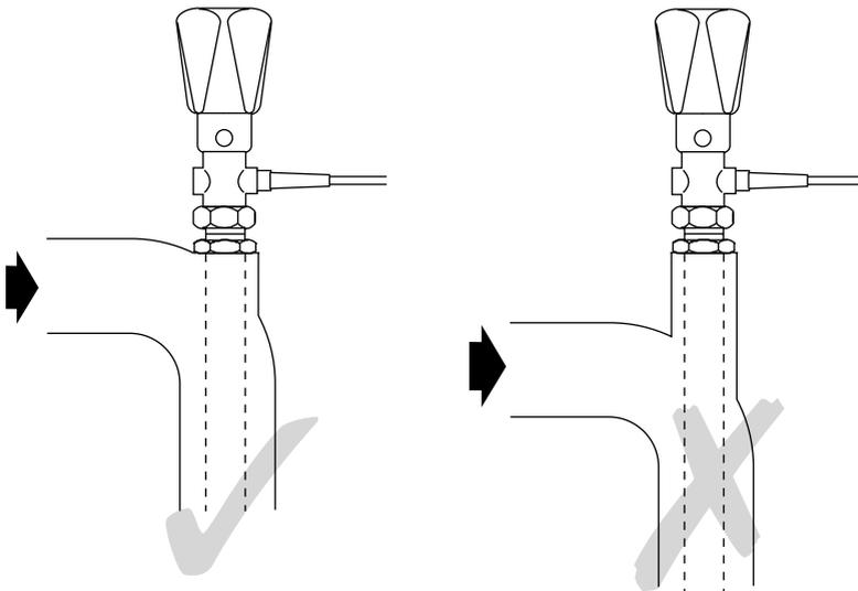
Fig. 1 Correct installation
