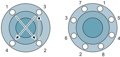
Flange bolts should be gradually tightened across diameters to ensure even load and alignment.
