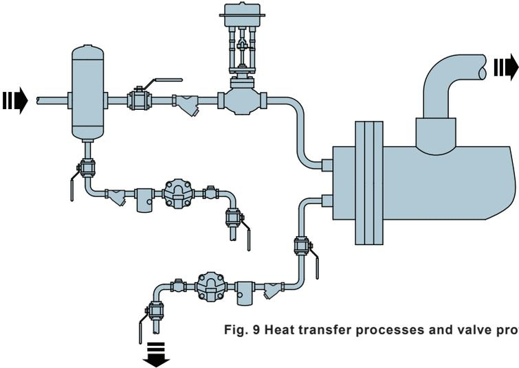
Fig. 9 Heat transfer processes and valve protection
