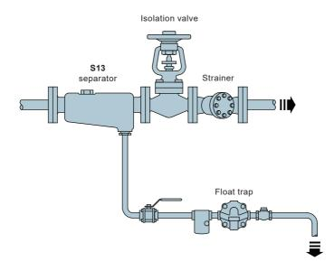
Fig. 6 Separator on a steam line
