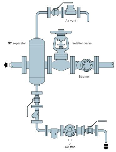
Fig. 8 Separator on a steam line
