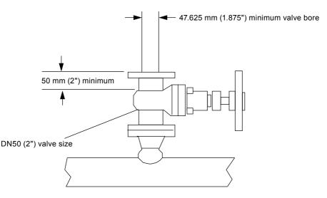
Fig. 3 Isolation valve requirements
