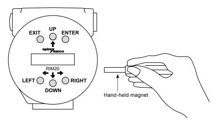
Fig. 47 Display/keypad commands
