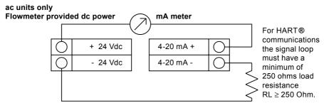
Fig. 30 Isolated 4-20 mA output using meter provided power supply
