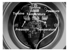
Fig. 53 Remote feed through board sensor connections
