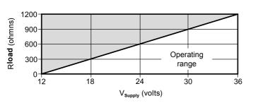
Fig. 27 Load resistance versus Input voltage
