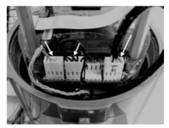
Fig. 52 Electronics stack sensor connections
