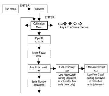
The Calibration menu contains the calibration coefficients for the flowmeter. These values should by changed only by properly trained personnel. The Low Flow Cutoff is set at the factory.
