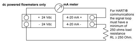
Fig. 29 Non-isolated 4-20 mA output using flowmeter input power supply
