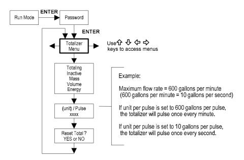
Use the Totalizer Menu to configure and monitor the totalizer. The totalizer output is a 50 millisecond (.05 second) positive pulse (relay closed for 50 milliseconds). The totalizer cannot operate faster than one pulse every 100 millisecond (0.1 second). A good rule to follow is to set the unit per pulse value equal to the maximum flow in the same units per second. This will limit the pulse to no faster than one pulse every second.
