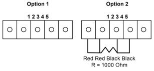
Fig. 42 Optional energy EMS RTD input wiring
