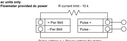
Pulse voltage = + Power voltage for meter
