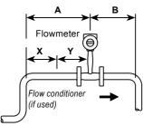
**Example 3**: Two 90° elbow before the RIM20 flowmeter out of plane (if there are three 90° bends present, double the recommended length) A Flowmeter
