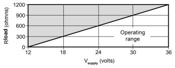
Fig. 15 Load Resistance Versus Input Voltage
