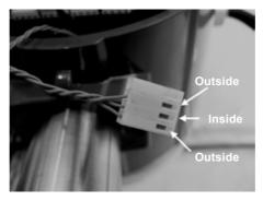
Fig. 54 Turbine Sensor Connector
