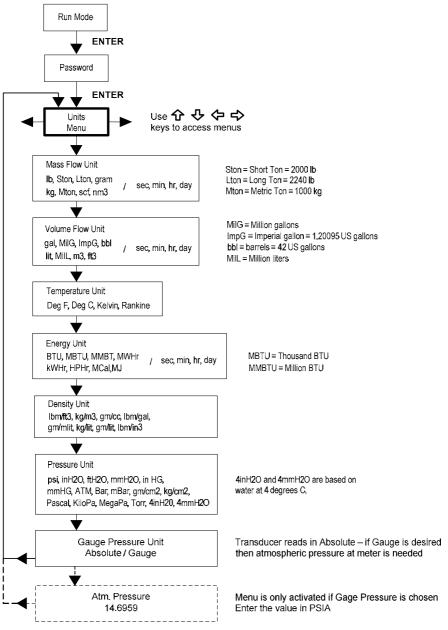
Use the Units Menu to configure the flowmeter with the desired units of measurement. (These are global settings and determine what appears on all screens.
