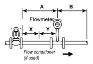
**Example 6**: If the regulator or valve is partially closed before the RIM20 flowmeter (If the valve is always wide open, base the pipe length requirements on fitting directly preceeding it)
