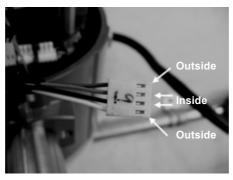
Fig. 56 Pressure Sensor Connector
