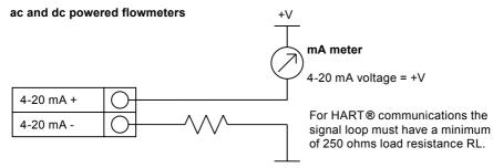
Fig. 28 Isolated 4-20 mA output with external power supply
