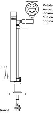
Rotate display / keypad in 90 degrees increments (maximum 180 degrees from original position)
