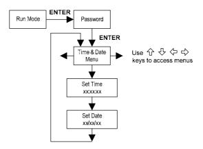
Use the Time and Date Menu to enter the correct time and date into the flowmeter's memory. The parameters are used in the Run mode and the alarm and system log files.
