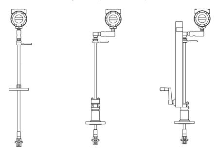
Fig. 1 Rotor Insertion multivariable Mass flowmeters
