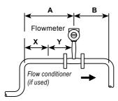
**Example 2 :** Two 90° elbow before the RIM20 flowmeter in one plane
