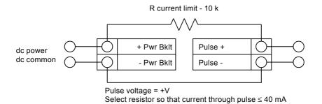
Fig. 17 Non-isolated pulse output using external power supply
