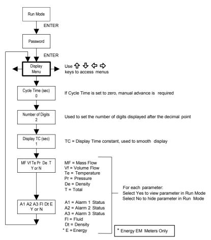
Use the Display Menu to set the cycle time for automatic screen sequencing used in the Run Mode, change the precision of displayed values, smooth the values or enable or disable each item displayed in the Run mode screens.
