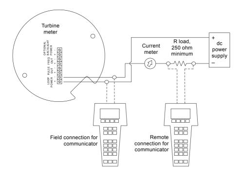
Fig. 48 Loop Powered Meter Wiring (HART)
