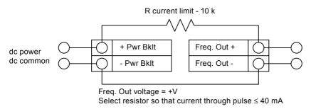
Fig. 32 Non-Isolated frequency output using input power supply
