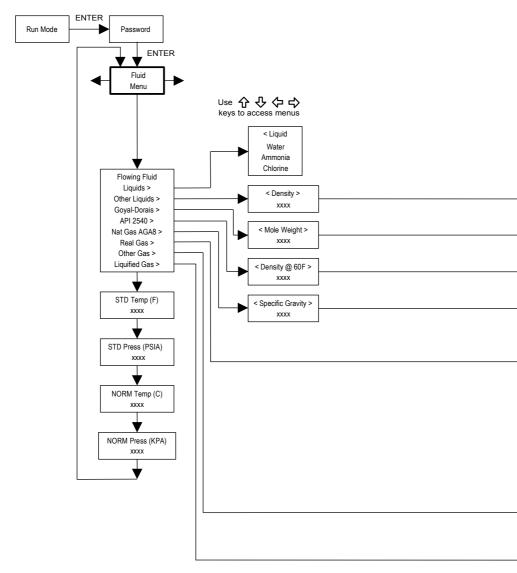
Use the Fluid Menu to configure the flowmeter for use with common gases, liquids and steam. Your flowmeter is pre-programmed at the factory for your application's process fluid. Reference Richard W. Miller, Flow Measurement Engineering Handbook (Third Edition, 1996), for definition and use of the Goyal-Doraiswamy equation and for the definition and use of the API 2540 equation. See Appendix C for Fluid Calculation equations.
