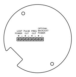
Fig. 13 Loop power wiring terminals
