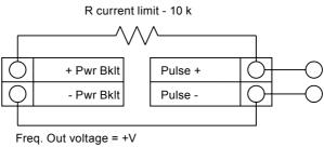
Select resistor so that current through pulse  $\leq$  40 mA
