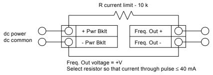
Fig. 19 Non-Isolated frequency output using external power supply
