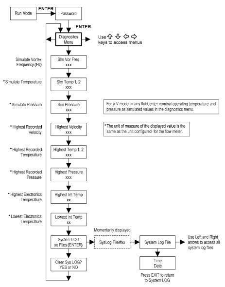
spirax sarco Use the Diagnostics Menu to simulate operation and review the system files. The system log files contain time/date stamped messages including: power on, power off, programming time outs, parameter faults, incorrect password entry and other various information relative to system operation and programming.
