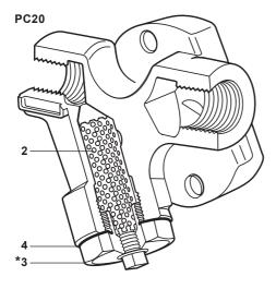
A blowdown valve, item 4, can be supplied as an optional extra for use on the PC20 for periodically removing pipeline debris.
