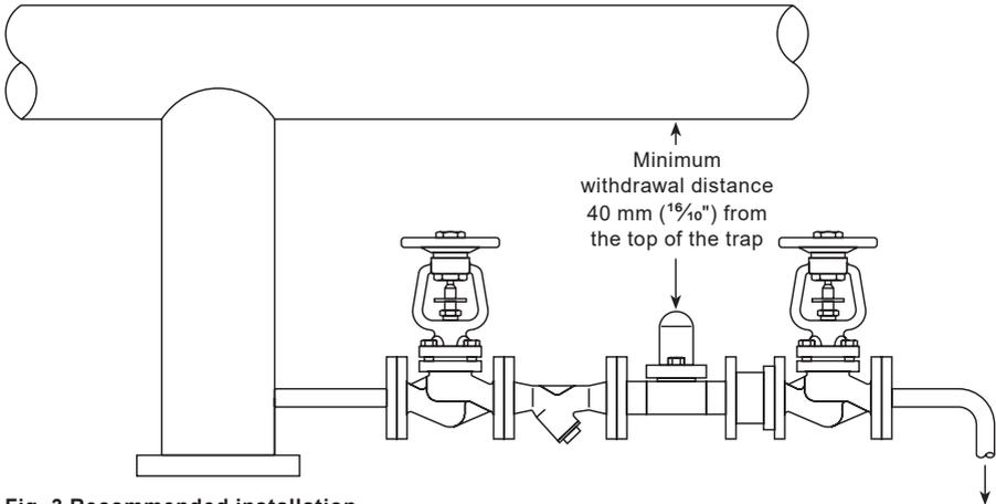
**Fig. 3 Recommended installation**
