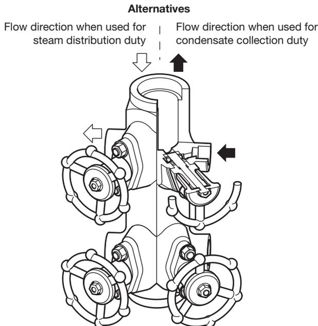
Fig. 1 Type MSC04-P socket weld version shown
