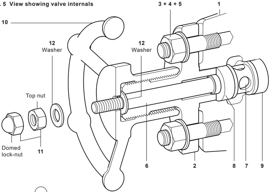
**Fig. 6 View showing valve internals extractor tool**
