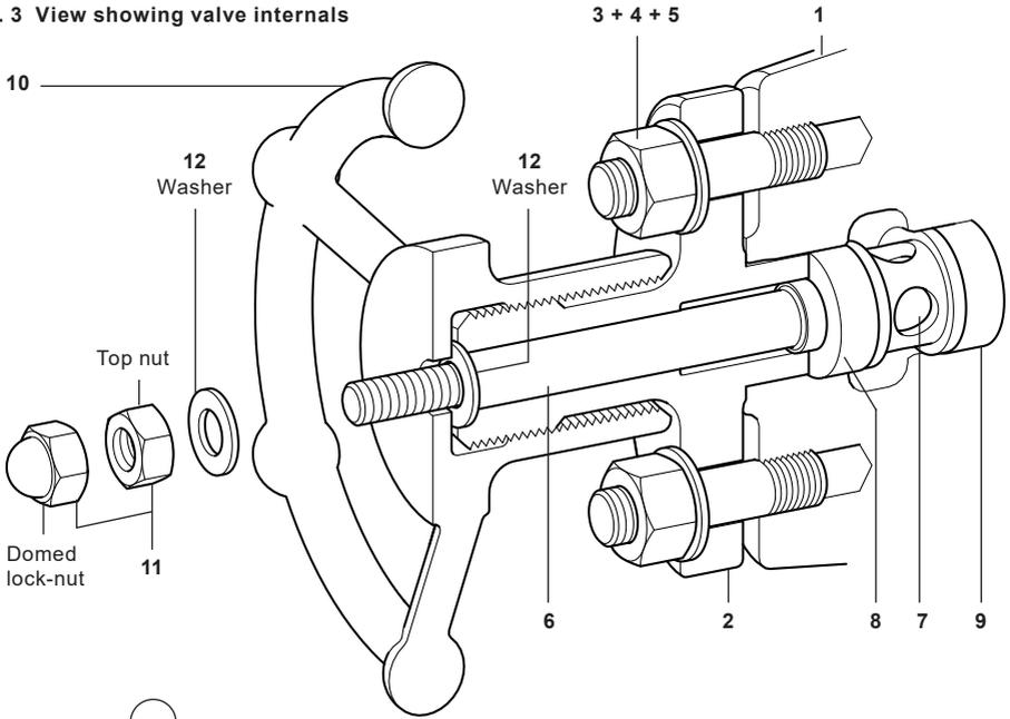
**Fig. 4 View showing valve internals extractor tool**
