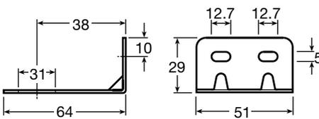
**Fig. 2** Type 8 mounting bracket
