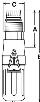
**Fig. 4** Withdrawal distance: **E** without bowl guard **E1** with bowl guard
