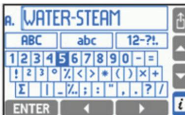
Horizontal and vertical arrow buttons move cursor along the whole screen. Left bottom button, depending on cursor position, can insert or delete a mark from edited text or change set of characters on keyboard. Button **i** is used to leave edition confirming a new text description. There is no possibility to interrupt edition and return to previous text.
