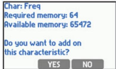
Pressing **REMOVE** button deletes all media (see Section 10.4.1.3 - Other liquid media) and all user's characteristics. The occupied memory volume is displayed next to the name on the list of characteristic tables. At the bottom of the screen the remaining free memory space is displayed. The database can store up to 16 characteristics.
