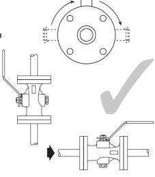
Fig. 3 Correct installation for gas service
