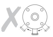
Fig. 2 Incorrect installation for liquid service
