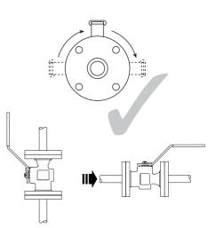
Fig. 3 Correct installation for gas service
