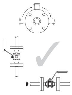
Fig. 3 Correct installation for gas service
