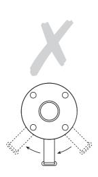
Fig. 2 Incorrect installation for liquid service
