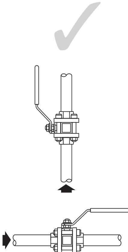
Fig. 3 Correct installation
