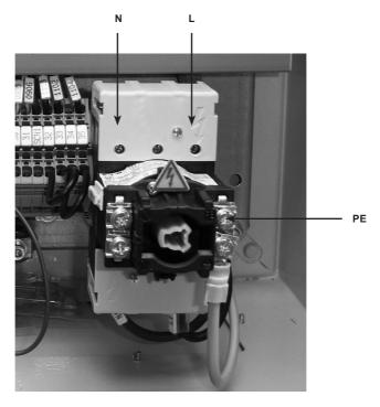
Fig. 6 Version with single-phase power supply (mod. "mCSG x00-xx1-...")
