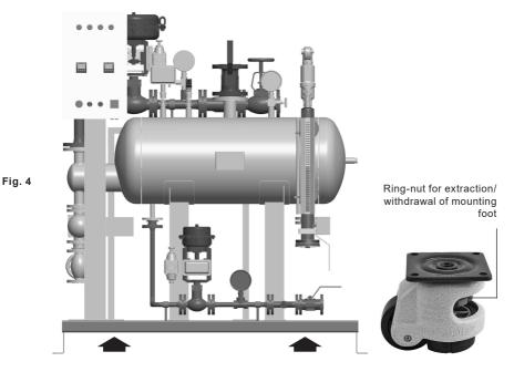
Do not use any eye-bolts of equipment on board the unit.
