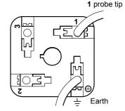
Fig. 4 Connector block removed from cable connector. Wired for use with an LC3000 controller as a high integrity, self-monitoring high level probe.
