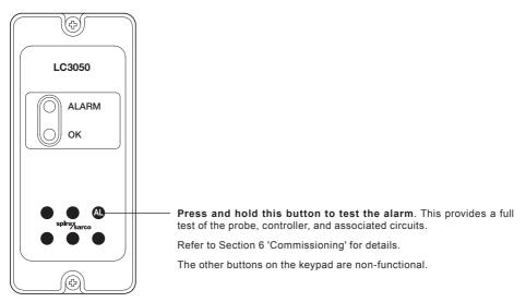
Fig. 1 Keypad button identification
