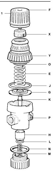
Replace complete bonnet assembly and retorque to 25 Nm, using a 42 mm spanner.
