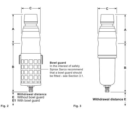
IP2M, IP2AM and IP2DM Monnier International Compressed Air Filter/Regulators
