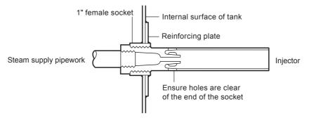
Fig. 5 IN15 injector - Typical installation through tank wall
