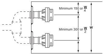
Fig. 7 Two injector layout
