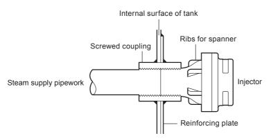
Fig. 3 IN25M/IN40M - Screwed coupling through tank wall
