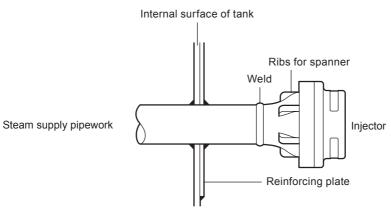
Fig. 4 IN25M/IN40M - Typical butt welded installation through tank wall (on a standpipe)
