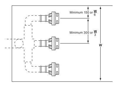
Fig. 8 Three injector layout
