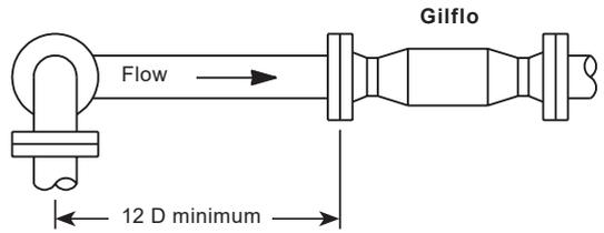
Avoid installing the Gilflo downstream of an actuated valve as rapid cycling of the valve could give rise to inaccurate results or damage the flowmeter (see Figure 6).
